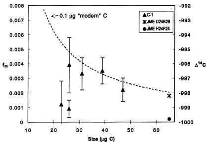
Fig. 7. Graphitization blank as measured for IAEA C-1 carbonate.
