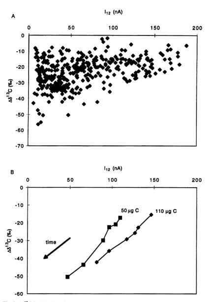
Fig. 5. A.  $^{13}$ C fractionation of HOxI and HOxII small samples as a function of the generated  $^{12}$ C ion current for all discrete time points. B.  $\Delta\delta^{13}$ C and  $I_{12}$  variation within samples as a function of elapsed measurement time.
