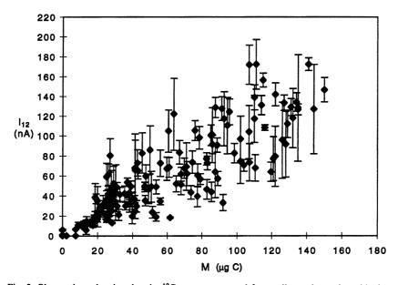
Fig. 3. Observations showing that the  $^{12}$ C current measured for small samples varies with size, according to the approximate relationship  $I_{12} = 0.9$ M. M = mass of carbon in micrograms;  $I_{12} = ^{12}$ C current in nanoamperes.
