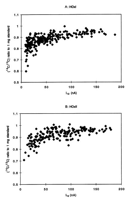
Fig. 4. Dependence of the measured <sup>14</sup>C/<sup>12</sup>C isotope ratios for HOxI (a) and HOxII (b) small samples on the generated <sup>12</sup>C ion current. Ratios have been normalized to average values obtained for HOxI and HOxII standards of conventional size.
