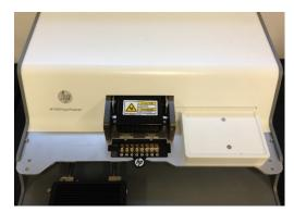
Please note that the D300 can dispense both aqueous and DMSO solutions, however ICCB-L only supports DMSO based dispensing using this unit.
