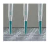
**Step 1**: Source Plate: Sample aspirated and pocket in tip fills to capacity (50 nl, 100 nl, or 250 nl).
